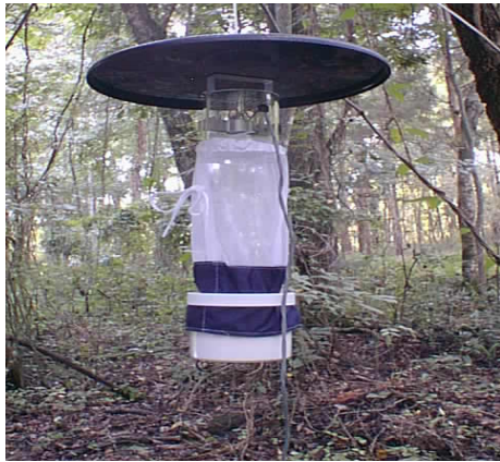
Figures 10 and 11. Left: CDC Miniature Light Traps. Right: CDC Gravid Trap. Source: ( http://home.acceleration.net/jwhock/pd_512.htm ).
